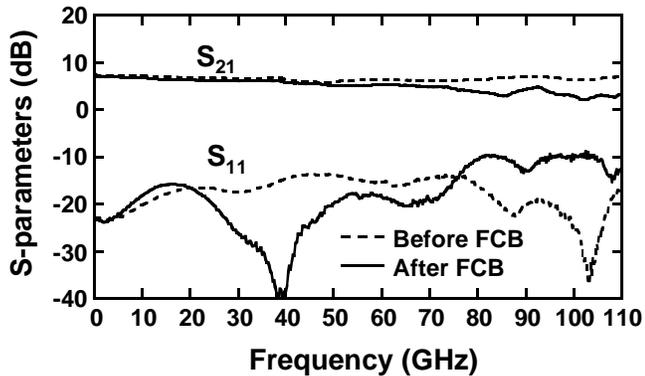
**Figure 11. Comparison of S-parameters before FCB and after FCB for seven-stage distributed amplifier. Solid line and dotted line indicate before and after FCB results, respectively**
