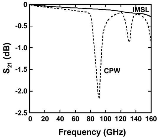
Figure 3. Comparison of simulated  $S_{21}$  characteristics of CPW and IMSL in distributed amplifiers. Solid line and dotted line indicate  $S_{21}$  of IMSL and CPW, respectively.
