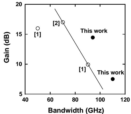
Figure 10. Comparison of gain versus bandwidth for distributed amplifiers.
