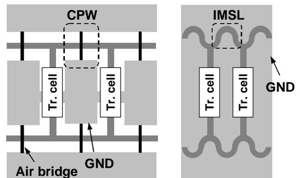
Figure 2. Comparison of schematic layout of distributed amplifiers designed with CPW and IMSL.
