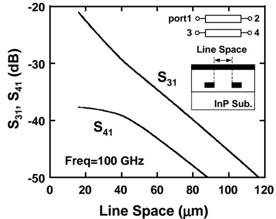
Figure 4. Simulated isolation characteristic of couple inverted microstrip lines at 100 GHz.
