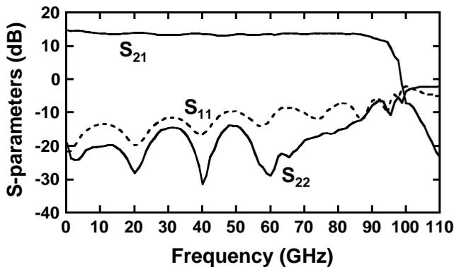
Figure 7. S-parameters of eight-stage distributed amplifier measured on wafer.
