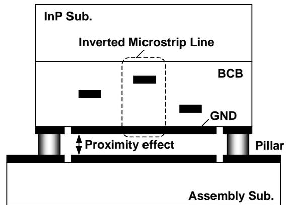
Figure 1. Schematic cross section of FCB multi-layer transmission line structure.
