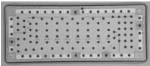
Figure 8. Microphotograph of seven-stage distributed amplifier. Chip size is 2.5 mm x 1.1 mm.
