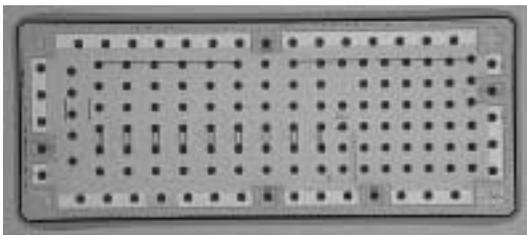
Figure 6. Microphotograph of eight-stage distributed amplifier. Chip size is 2.5 mm x 1.1 mm.
