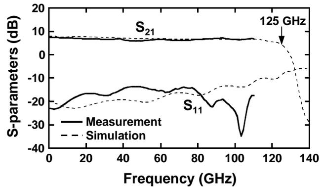
Figure 9. Comparison of measured and simulated S-parameters for seven-stage distributed amplifier. Solid line and dotted line indicate measured and simulated results, respectively.
