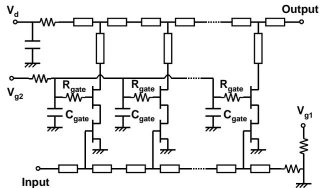
Figure 5. Circuit diagram of distributed amplifier.
